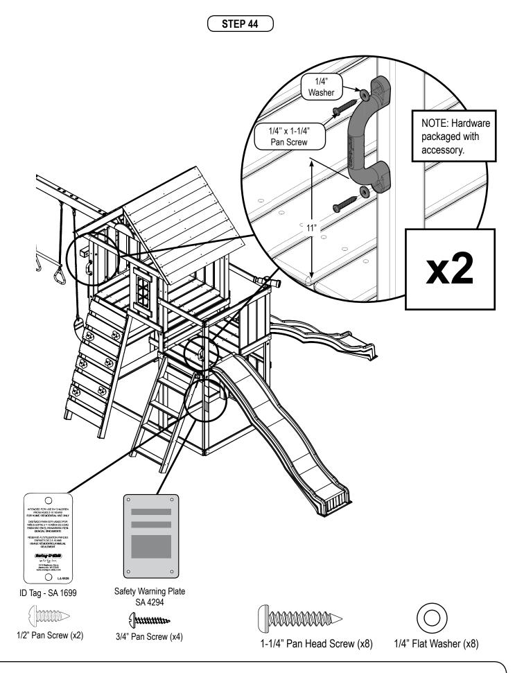
1. Attach Safety Handle, Plate and I.D. Tag, as shown.
