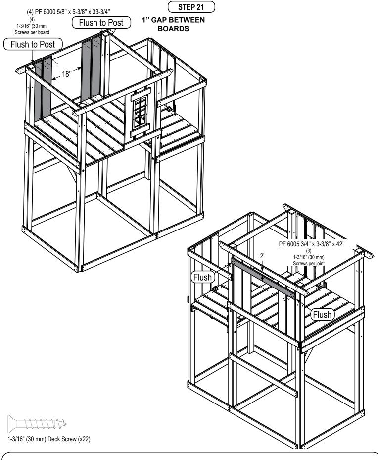
1. Install Barrier Boards as shown.
