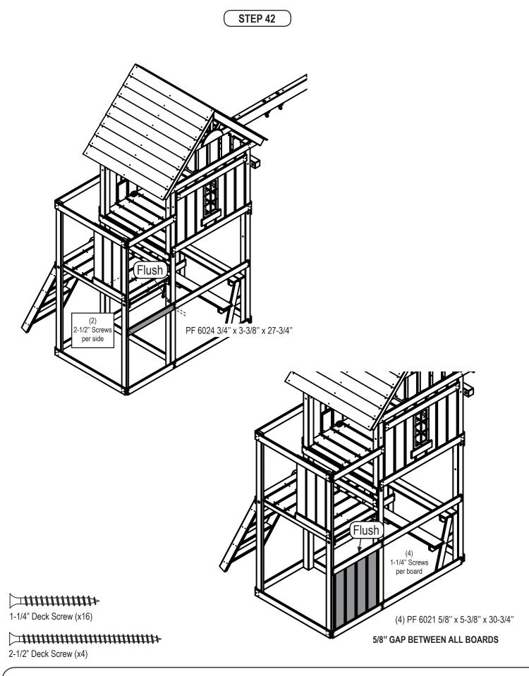
1. Install Barrier Support and Barrier Boards as shown.
