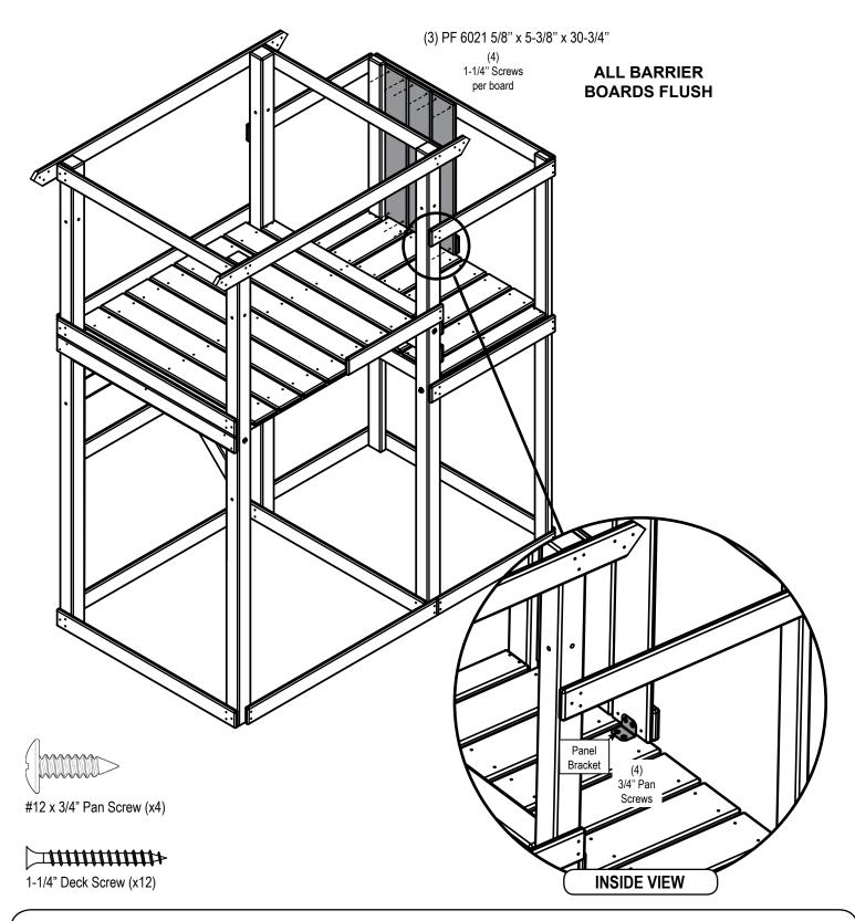
1. Install Barrier Boards as shown.
