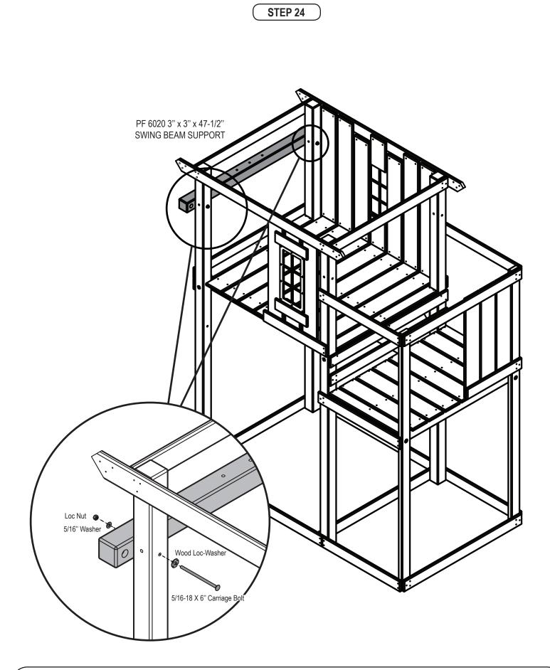
1. Install Swing beam support as shown.
