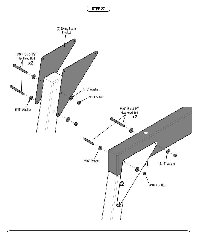
1. Attach Swing Beam Bracket to A-Frame & Swing Beam as shown.
