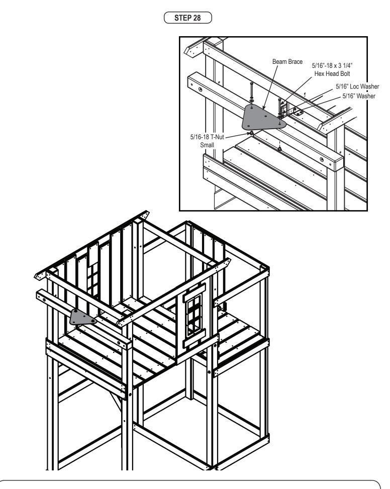
1. Install Swing Beam Brace as shown.
