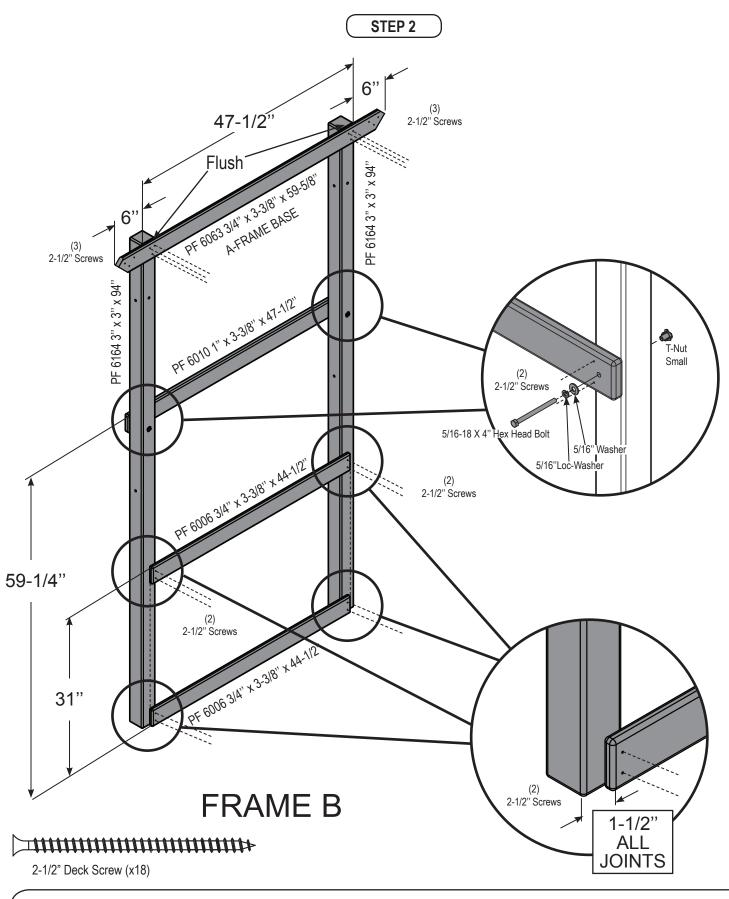
1. Assemble Frame B as shown above. **Note:** Tap each T-Nut into its pre-drilled hole until the metal tangs sink fully into the wood.
