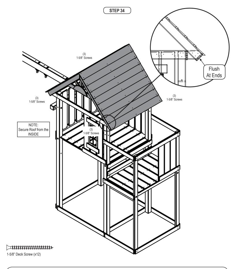
1. Attach Roof Frame to Tower as shown. **NOTE:** Secure roof from inside the tower.
